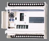
Programmable Logic Controller (PLC)
