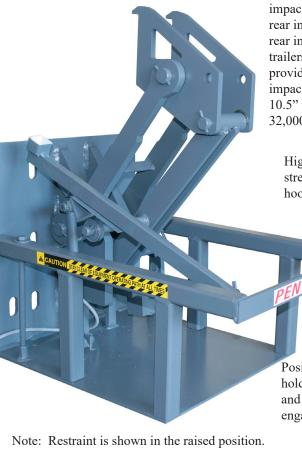
10-1/2 inch lowered height facilitates "no impact" operation. Accommodates vehicle rear impact guards and meets 1998 NHTSA rear impact guard bar regulations for trailers. The MFRAL32 Vehicle restraint provides a 10.5" lowered height. It is a nonimpact design with an operating range of 10.5" to 28.5" and a restraining capacity of 32,000 lb.
