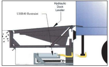
**Benefits:** The "under dock" position of the restraint protects the restraint from adverse conditions on the outside of the dock area. Only the restraint arm is exposed to the external adverse elements at the loading dock. The concerns highlighted below are eliminated.
