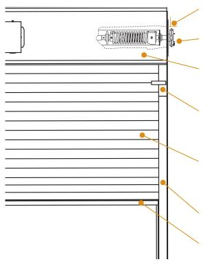
**BRACKETS** - Steel with powder coating to match curtain. Bolt to guide assembly and support counter-balance shaft and curtain.
